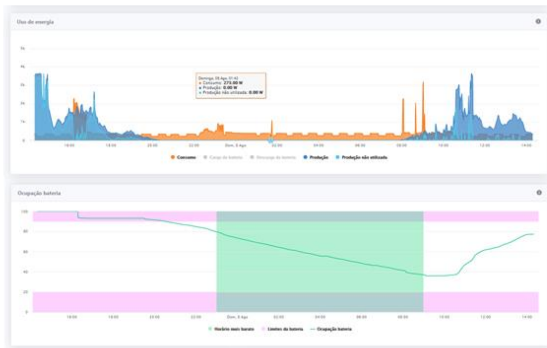
Figure 19. Interface providing information about (on the top) load flows - consumption, PV production, and PV surplus - and (on the bottom) State of Charge (SOC) of the BESS.
