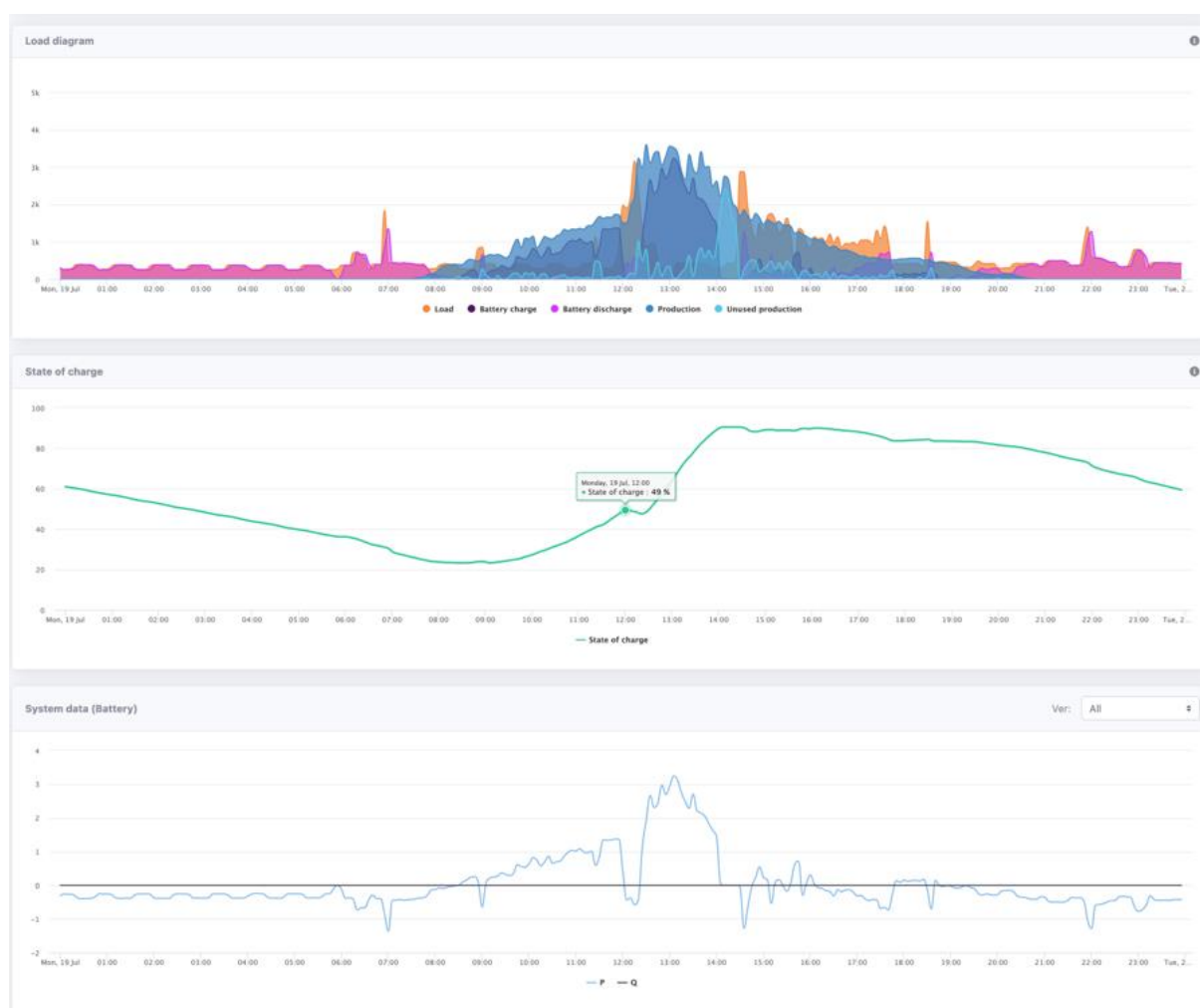
Figure 5. Combination of UI widgets to provide a dashboard with information about storage control. On the top the load flows (including battery charge and discharge), in the centre the battery SOC, and on the bottom the active and reactive power as seen from the battery inverter.
