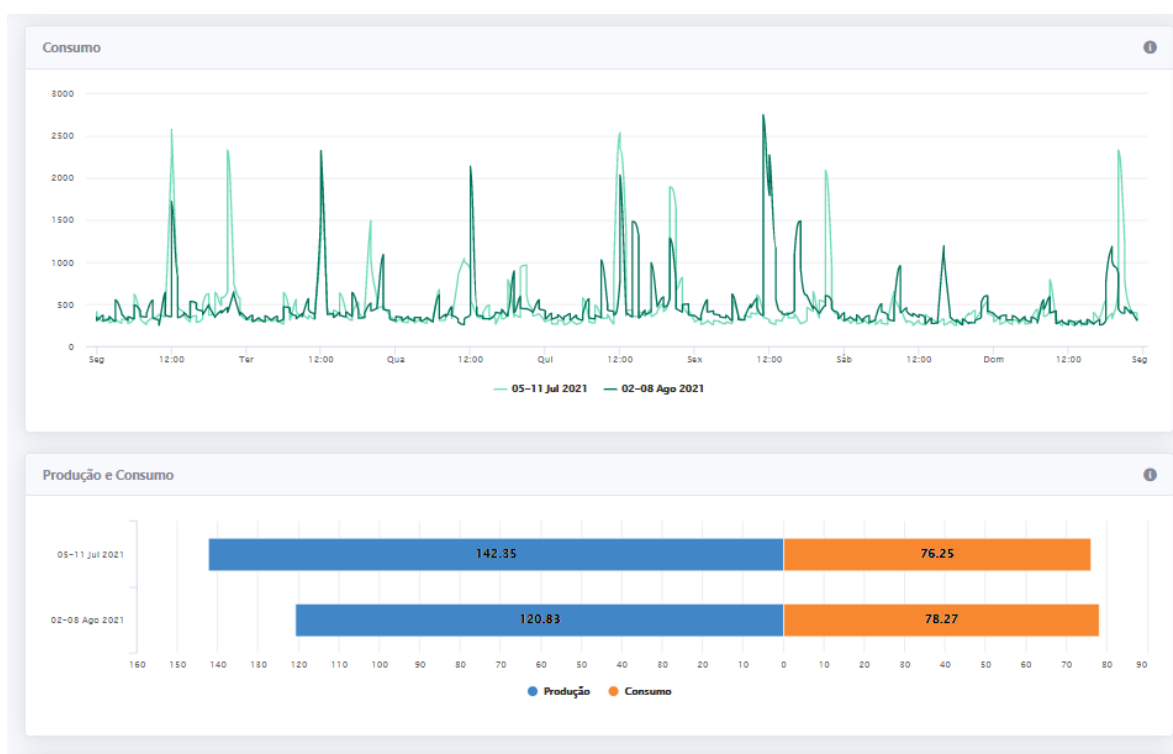
Figure 17. Combination of UI widgets to provide a dashboard for UPACs comparing production and consumption data from two different weeks.
