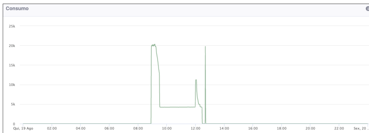
Figure 39: Daily load for charging point 6. The smart charging command is visible between 9 and 12:00 approximately
