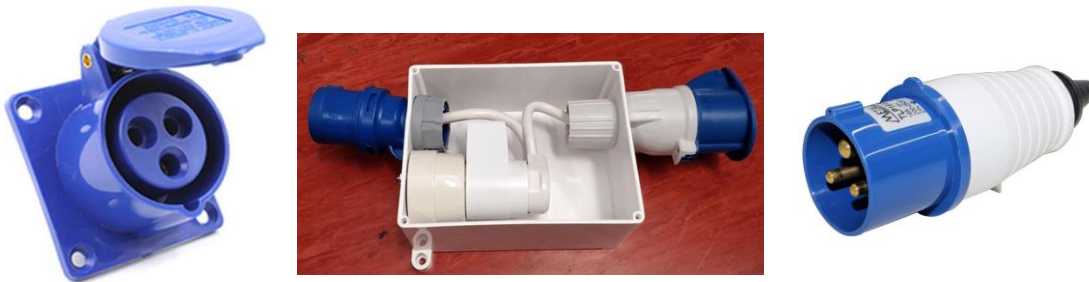
Figure 2: Different components part of the Control Module. Left: CE16 female socket; Middle: control module with the smart-plug fitted; Right: CE16 Male socket
