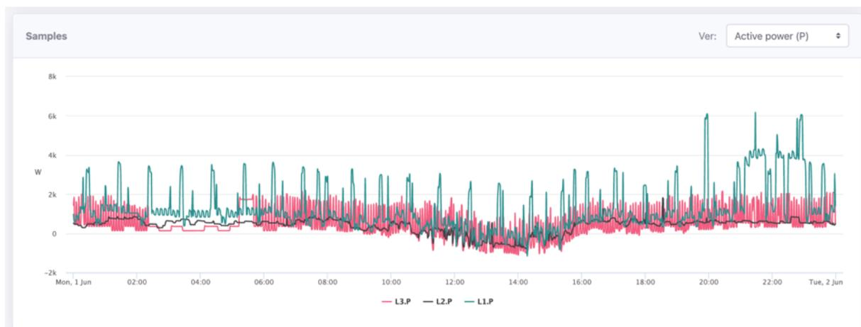
**Figure 3.20: One days of minutely averages of active power for the three phases in UPAC 8.**
