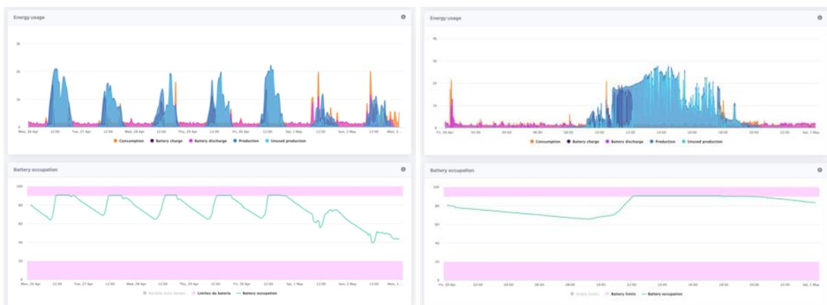
Figure 3.7: Energy flows and battery SOC for one week (left), and one day (right) in April for UPAC 2.
