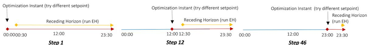
Figure 4.3: Illustration of the receding horizon optimization procedure.
