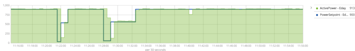
Figure 5: Graph Illustrating the setpoint and active power of the Eday turbine. In this example, highlighting two periods during which the turbine was curtailed
