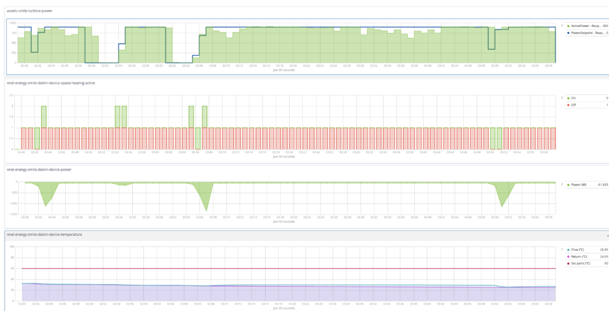
Figure 21: Curtailment events and heat pump response in Type 3 system
