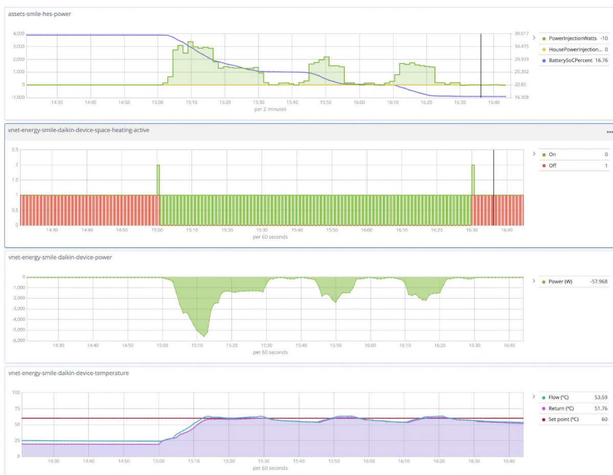
Figure 26: Lithium Balance battery discharges stored energy from a previous curtailment event to match the power consumption of the heat pump
